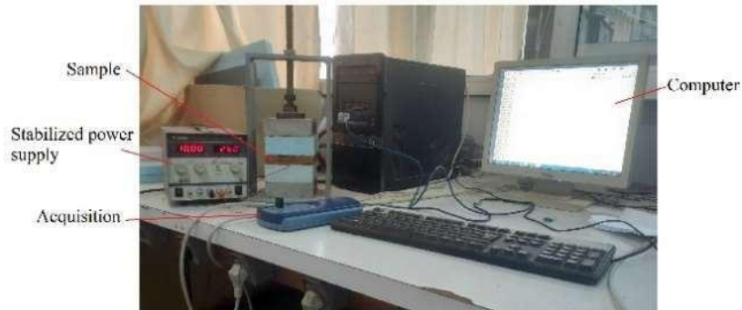
Fig.3 Schema of the experimental asymmetrical hot plate device (Bodian, 1987).
